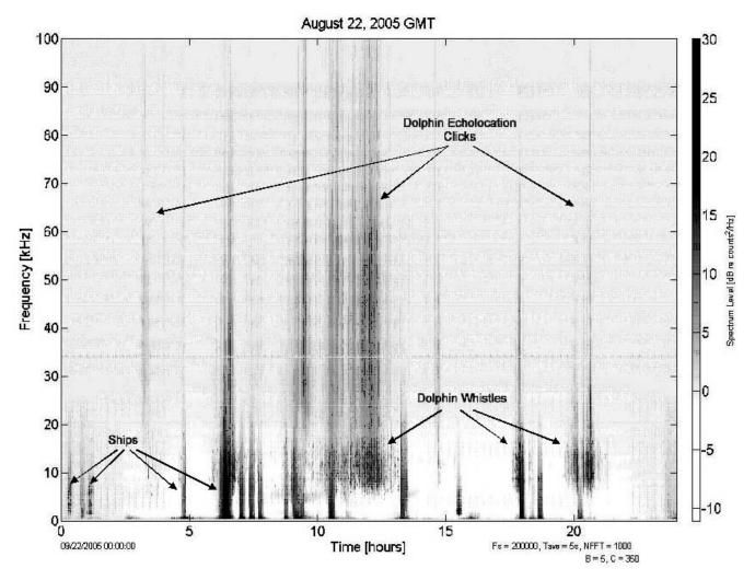
Figure 8. Long-term spectral average of HARP data collected at CalCOFI station 82.42. One days' worth of data is represented, showing the presence of delphinid echolocation clicks and whistles, as well as noise from ship passings.
